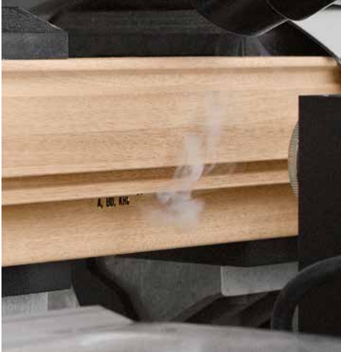
Laser device for marking work-pieces.
