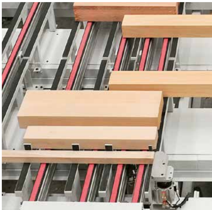
Central reference stop for the work-pieces positioning on the loading system.
