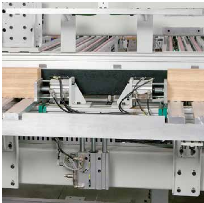
The centering devices ensure the correct work-pieces alignment on the worktable.
